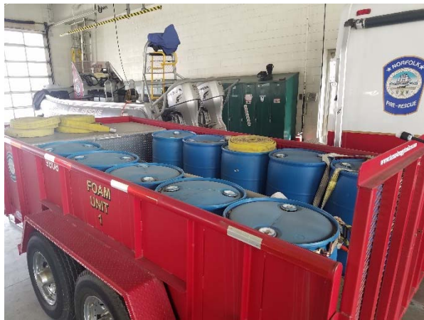
Photograph 55. View of stored fire suppressant foam stored within 50-gallon containers.
